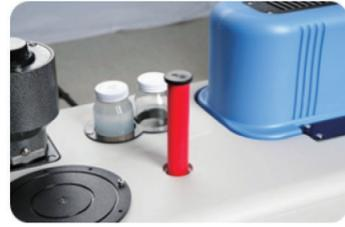
▶ If the red level indicator is raised at the upper part of the pre tank, replace the filter as it indicates that the filter is blocked.
