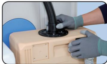
▲ Fasten the Clamp after connecting the hose.
